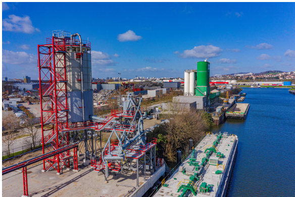
The movable arm has two main pivots in order to feed barges in only two manoeuvres.
