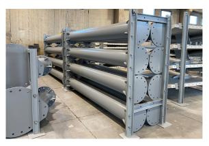
A complex system of racks and packaging has been developed to prevent items from damage during sea transportation.
