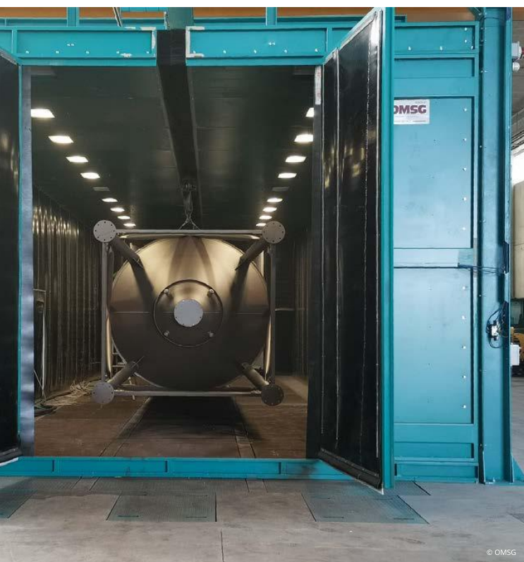
The inside of the shot blasting plant: the cabinet is equipped with 16 turbines, each with a power of 7.5 kW.
